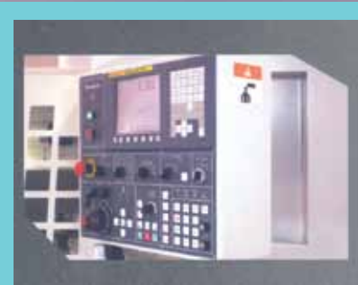
The ergonomically rotating control panel box design provides convenient use
