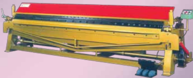
UNIVERSAL HYDRAULIC PRESS BRAKE SERIES OF MODAL AVAILABLE TABLE LENGTH FROM: 1260mm - 2000mm CAPACITY FROM: 3.2mm ONWARDS
